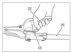
With the lock released, grip the adjustment lever [5] to change the angle of the cutter bar.
