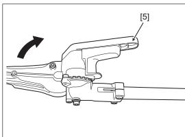
At the adjusted angle position, return the lock lever. (Engage the pin [3] of the lock lever with the hole.)
