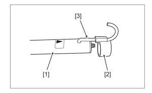
Insert the pipe cap [2] into the shaft tube [1].
