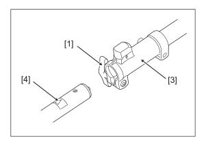
Align the boss (protrusion) [2] at the end of the pipe with the slit of the joint case [3], and insert it to the label [4] position.
